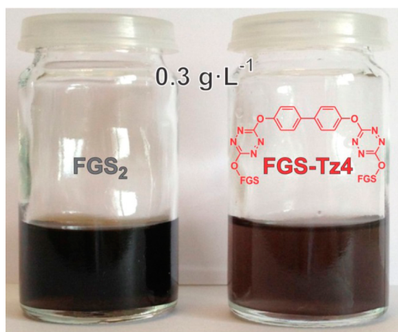
Figure 1. Pictures of 0.3 g·L -1 suspensions of unmodified FGS 2 (left) and grafted FGS-Tz4 (right) in PC.
