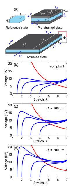
FIG. 1. (a) Schematics of DE actuator in different states. (b)–(d) Mechanical response of DE membranes with electrodes of different stiffness. The red curves correspond to the electric breakdown limit of 200 MV/m. (b) Perfectly compliant electrodes, (c) and (d) solid electrodes,  $H_0 = 1 \text{ mm}$ .
